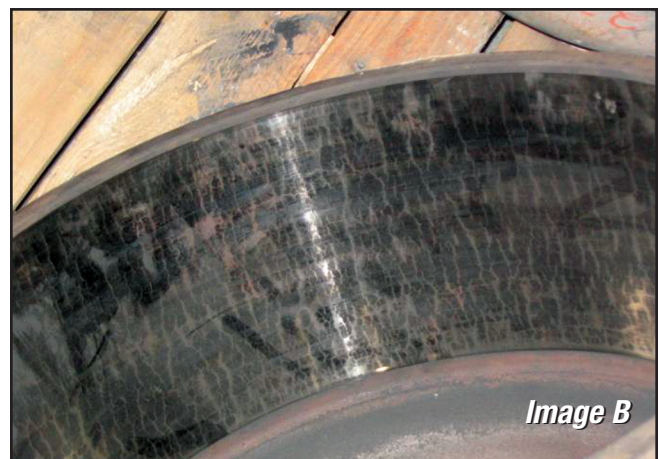
Heat checking and martensite on the brake surface
